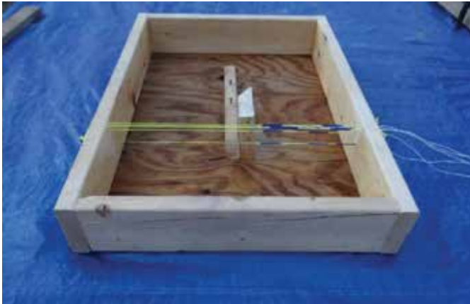
Fig. 5: Test slabs were constructed using 2 x 3 ft x 5-1/2 in. deep (610 x 915 x 140 mm) forms containing thermistors spaced at different depths (1/8, 1/4, 1/2, 1, and 2-1/2 in. [3.2, 6.4, 12.7, 25.4, and 63.5 mm]) from the top
