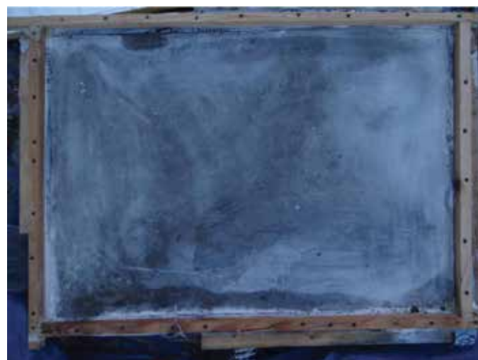
Fig. 7: After 1-1/2 hours, the ponded curing water was removed, the slab surface was checked for cracks, and then 36°F curing water was reapplied to the concrete surface. No cracking was observed during or after drying of the surface
