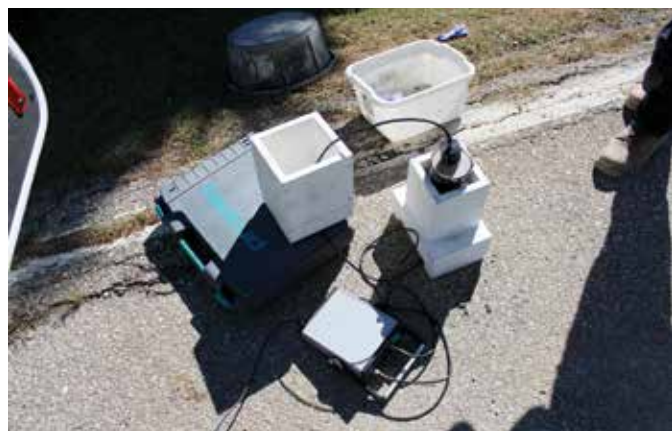
Fig. 8: UPV test setup with sample and transducers in a wooden frame for stability
